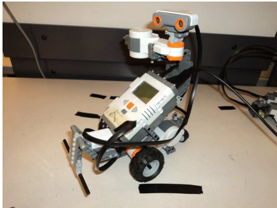
Fig. 11.2 Tribot configuration for the wall avoidance experiment.
