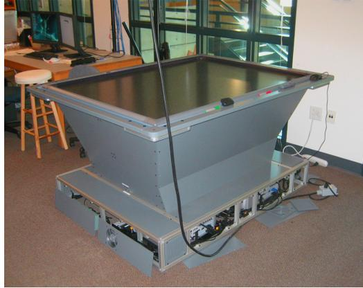
Figure 4.3: SMART Technologies prototype tabletop display at Dalhousie University has a 77-inch display which supports up to two simultaneous inputs.
