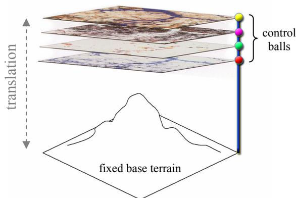
Figure 2: Multiple 2D thematic layers in a combinational display with a 3D base terrain. Vertical translation of layers is set with the associated control balls.
