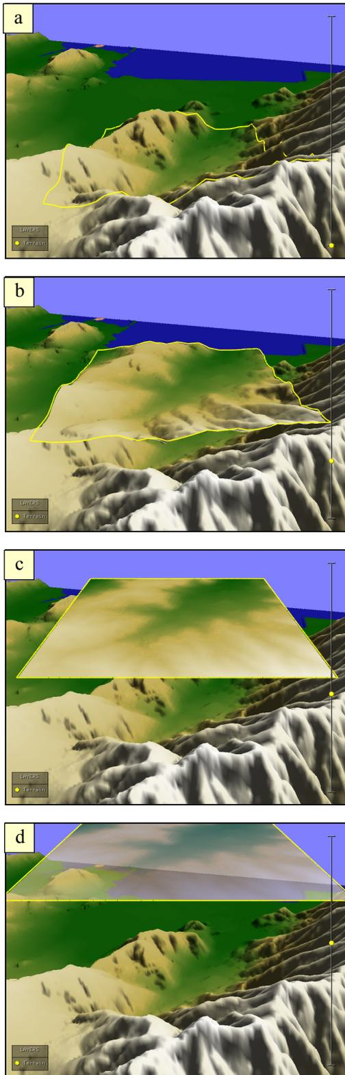
Figure 4: The layer is shown gradually rising from image a to image d. As the layer rises it morphs into a flat plane. Image c shows the layer completely flat at level  $m$ . Above level  $m$ , the layer becomes increasingly transparent as shown in image d.
