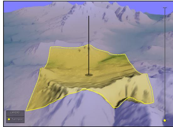
Figure 3: Layer shown as a terrain geometry clipped with 4 perpendicular clipping planes equidistant from the centre (shown as black vertical line). The original terrain is shown faded to highlight the relationship.
