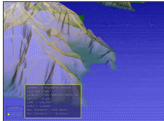
Figure 1: A regular grid DEM shown in wire-frame mode.
