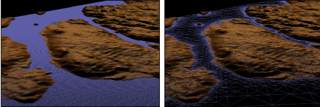
Figure 3. High-density wireframe rendering without (left) and with (right) level-of-detail.
