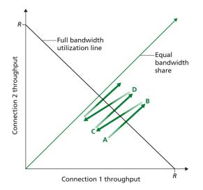
Suppose that instead of a multiplicative decrease, TCP decreased the window size by a constant amount. Consider the case where both connections get the same constant decrease and the case where one connection gets a bigger constant decrease than the other. Would the resulting AIAD converge to an equal share algorithm? Justify your answer using two diagrams (for two cases) similar to the figure above.
