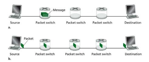
Consider a message that is  $7.5 \times 10^6$  bits long that is to be sent from source to destination as in the figure. Suppose that each link is 1.5 Mbps. Ignore any propagation, queuing or processing delays.
