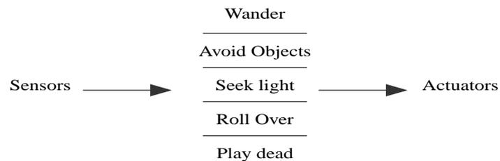
**Figure 3-3.** Decomposition of a mobile robot control system based on task achieving behaviours (Brooks 1986)
