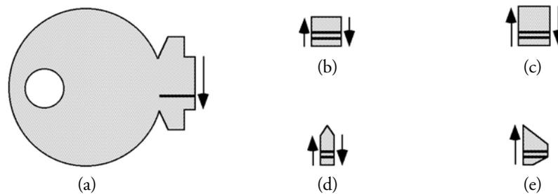
**Figure 2.7:** Components of a key solid with two possible bit cuttings.
