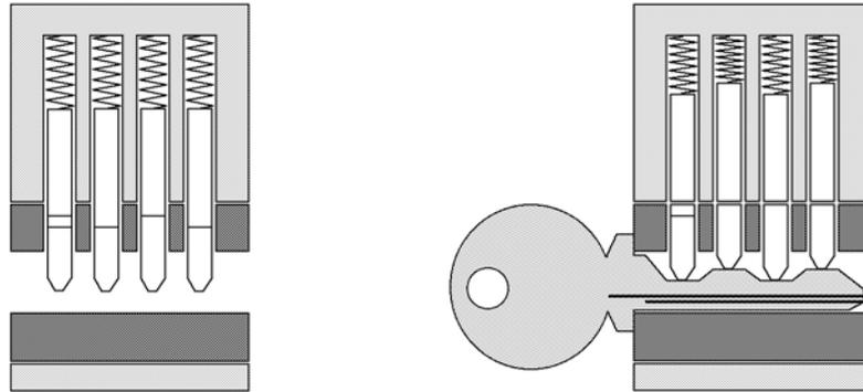
**Figure 2.13:** A side view of a lock and one of its keys.
