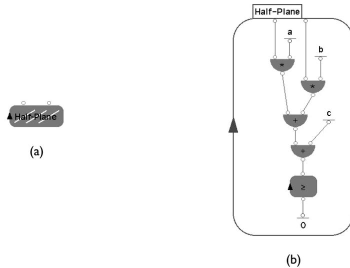
**Figure 3.2:** A constraint cell (a) and its specification (b)
