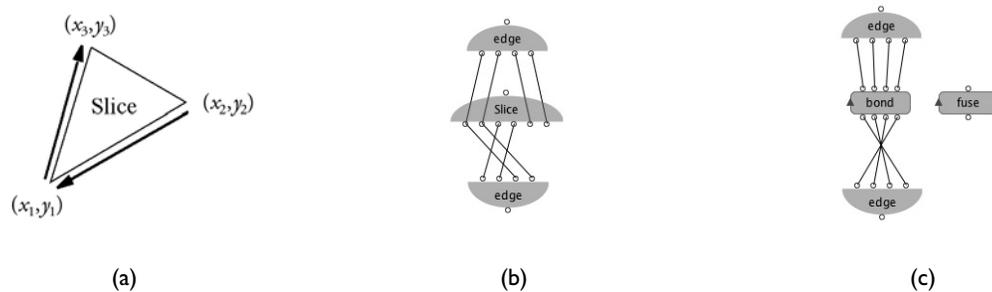
**Figure 6.2:** **Slice** solid, and LSD representations of **Slice** and the bond operation
