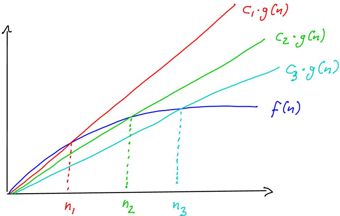
So, no matter the constant we multiply  $g(n)$  with, there always exists an input size beyond which  $f(n)$  will "dive below" that scaled version of  $g(n)$ .
