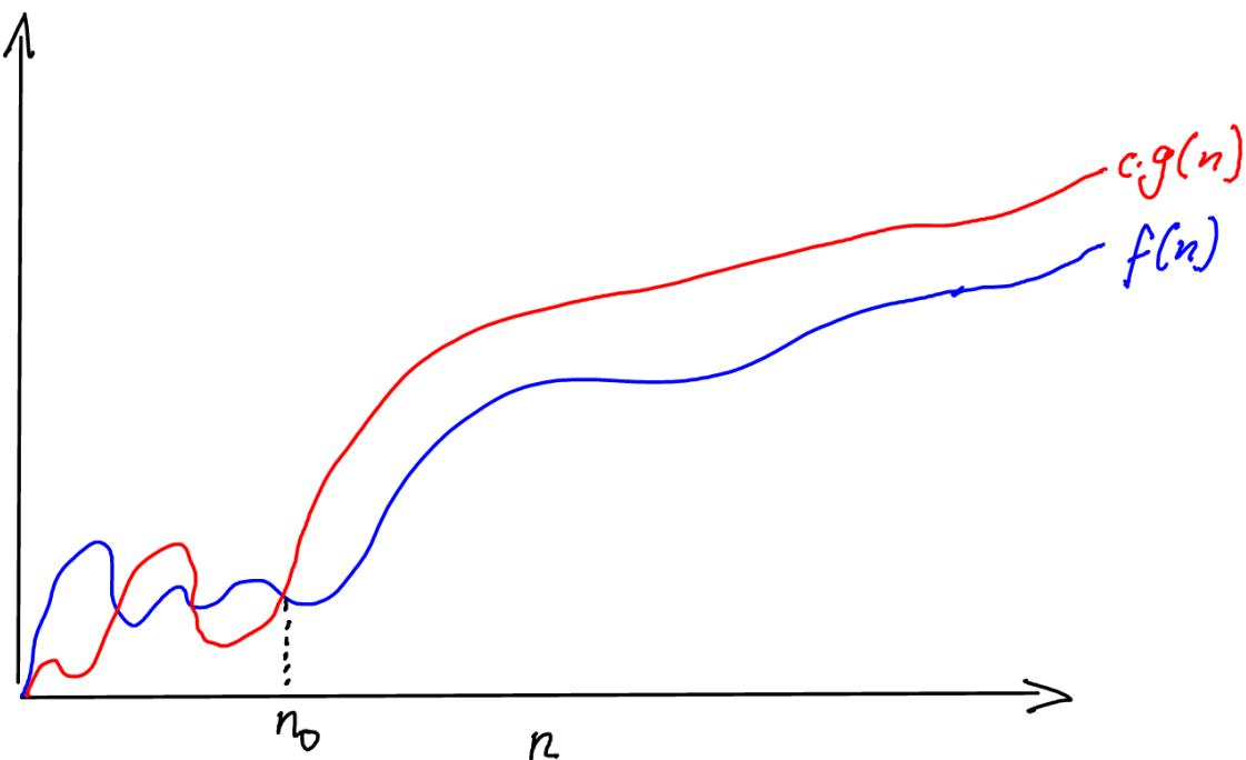
$f(n) \in \Omega(g(n)) \Leftrightarrow \exists c > 0, n_0 > 0 \forall n \geq n_0 : f(n) \geq c \cdot g(n)$
