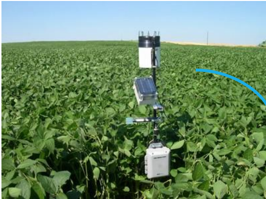
Fig 1: Remote monitoring equipment (Source: NDSU )
