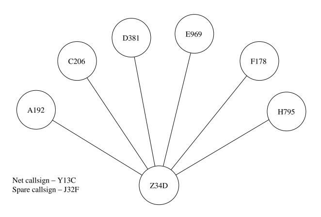
The following diagram shows connectivity between stations. Note that callsign B420 is a member of another net and is only able to receive messages relayed from callsign D381.
