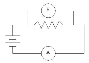
And, in a final bold stroke, I note that if the battery is 6 volts and the resistor 6 ohms, then one ampere of current flows in the circuit:
