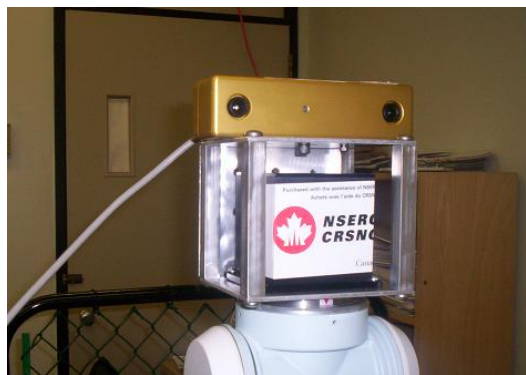
Figure 1: The Bumblebee stereo camera from Point Grey Research mounted at the tip of the PA10-7CE robot arm.
