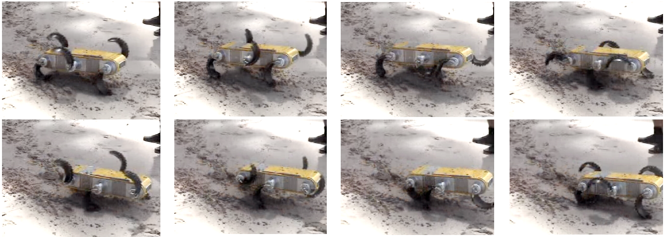
Figure 2. Eight snapshots of the AQUA vehicle walking along the beach. The individual frames should be viewed in a left to right, top to bottom order. AQUA maintains a statically stable gait while walking.
