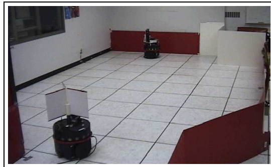
Figure 1: The two robots exploring a laboratory. In the lower-left one robot carries a three plane target, on the upper-right a second robot is mapping.
