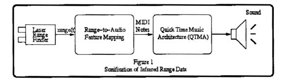
Two modes of operation have been defined. The *proportional* mode (range to audio feature mapping) provides the user with a general knowledge regarding both the close-by and distant surroundings through the detection of objects, doorways, depth discontinuities, etc. The *derivative* mode (temporal derivative of range to audio feature mapping) is used to obtain the greater detail necessary for shape and pattern detection.
