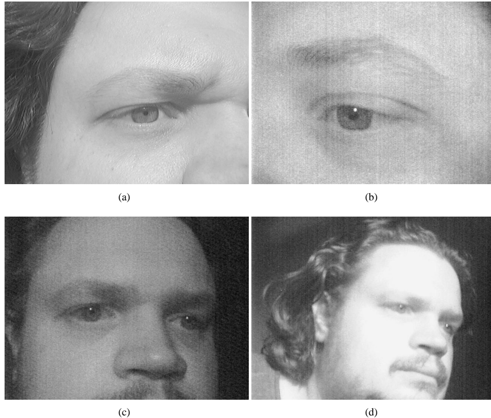
Figure 4: Sample images from Logitech QuickCam with film negative infrared transmission filter and built-in infrared block filter. a) Using the sun as a source on a bright, clear day. b) Using a normal desk light as a light source. c) Using a heat lamp as a source. d) Using a heat lamp as a source with Logitech driver's Low Light mode.
