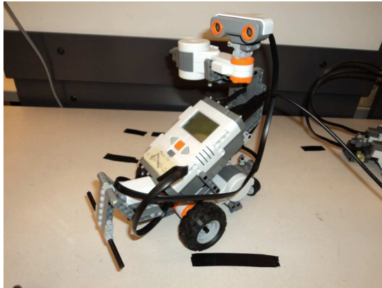
Fig. 11.2 Tribot configuration for the wall avoidance experiment.
