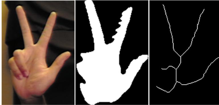
Fig. 12. Successful detection of a 3-finger hand gesture.
