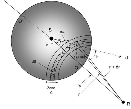
Fig. 3. Fresnel zone geometry.
