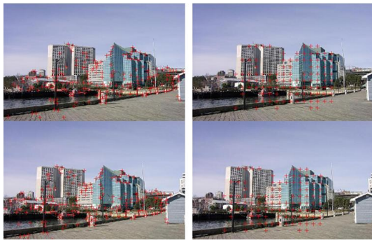
Figure 1 Feature correspondences on images. Right images display the corner features with red cross, and left are the evenly distributed features.
