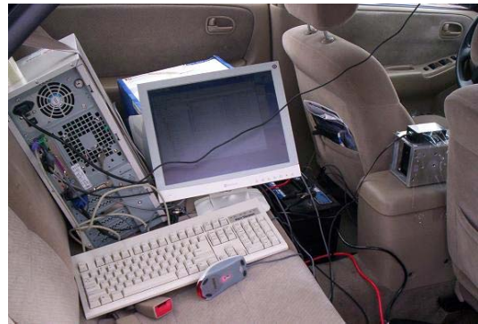
Fig. 6. Experimental setup for land vehicle navigation with IMU, GPS and Digital Compass
