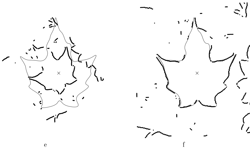
Figure 9.4: (a) An image of a leaf shape from which a contour curve model is derived. (b) An image of the same leaf shape in a cluttered background. (c) The derived curve model from the image in (a). (d) The edge points extracted from the image in (b). (e) The points are initially registered to the model by a moment-based global procedure. (f) The points are matched to the model as the matching algorithm recovers the geometric transformation.
