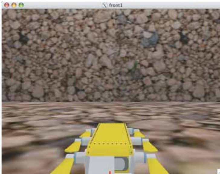
Figure 2. A “co-pilot” view from one of the AQUA simulators. Researchers can use these simulators for task rehearsal as well as hydrodynamic simulation of gait and fin design.
