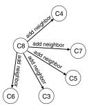
Fig. 4. Discover alive peers and form mesh; mesh degree depends on number of peers.
