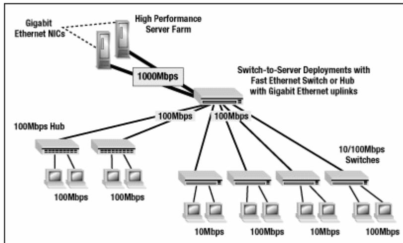
Figure 4. Switch-to-Server Deployment
