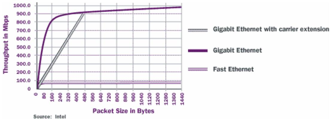
Figure 6. Gigabit Ethernet Performance Simulation
