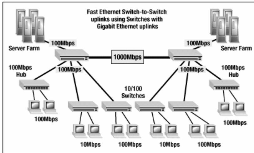
Figure 3. Switch-to-Switch Connection
