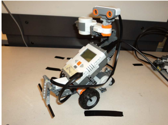
Fig. 10.5 Tribot configuration for the wall avoidance experiment.
