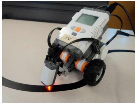
Fig. 3.1 Basic Lego Robot with microprocessor, two motors, and a light sensor.
