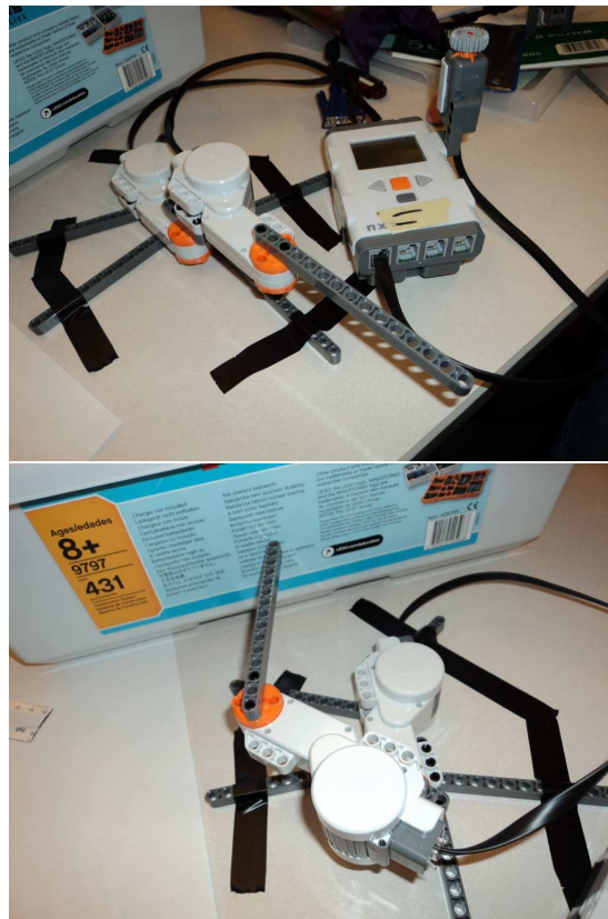
Fig. 3.3 (A) Robot arm with two joints. (B)
