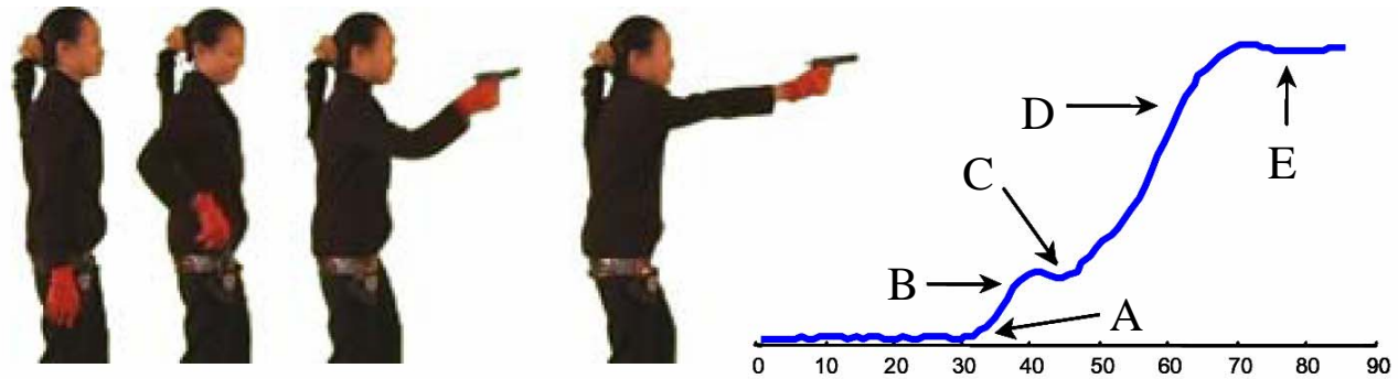
Figure 10. Stills from a video sequence; the right hand is tracked, and converted into a time series: A) Hand at rest: B) Hand moving above holster. C) Hand moving down to grasp gun. D) Hand moving to shoulder level, E) Aiming Gun.
